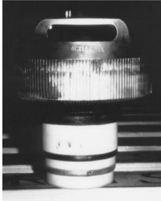
**Figure 13.** A 4CX15000A tube showing signs of external arcing.
