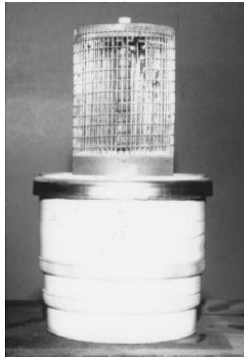
**Figure 12.** The interior elements of a 4CX15000A tube that had gone to air while the filament was lit.
